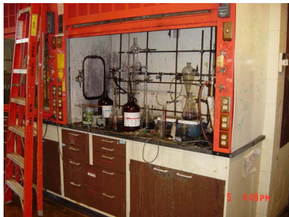
Figure 1. Fume hood where the fire originated (in corner), during a recrystallization with acetone and petroleum ether.
