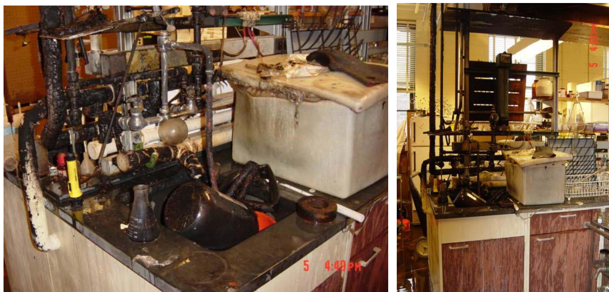
Figure 2. The (flaming) 4-liter solvent bottle was placed in sink outside of fume hood. The fire continued to burn, and could not be put out by handheld extinguishers. The automatic sprinklers were eventually activated.
